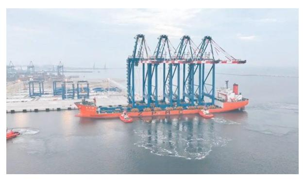
Baltic Hub's T3 terminal is set to receive four state-of-the-art ship-to-shore (STS) cranes, arriving directly from China. Each crane stands over 96 meters high (140 meters with the boom raised) and weighs approximately 2,000 tonnes. The cranes embarked on a 16,115-nautical-mile journey, circumnavigating Africa.
